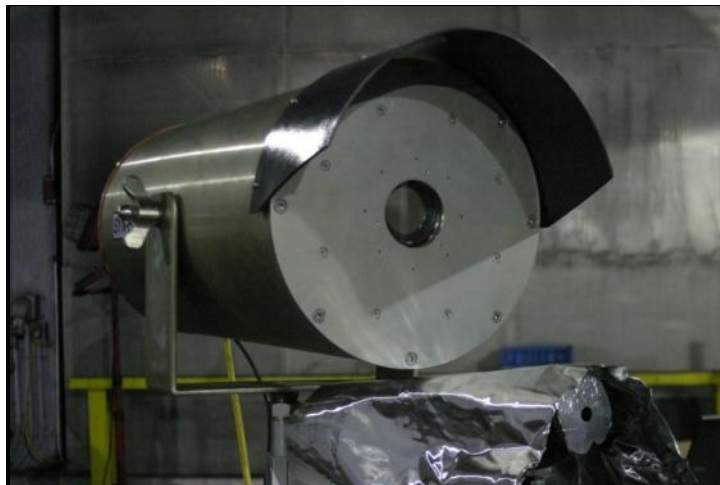
Figure 4-18: The SC7600 MWIR inside protective enclosure (center) and the SC655 LWIR camera protected by aluminum foil (lower right hand corner)
