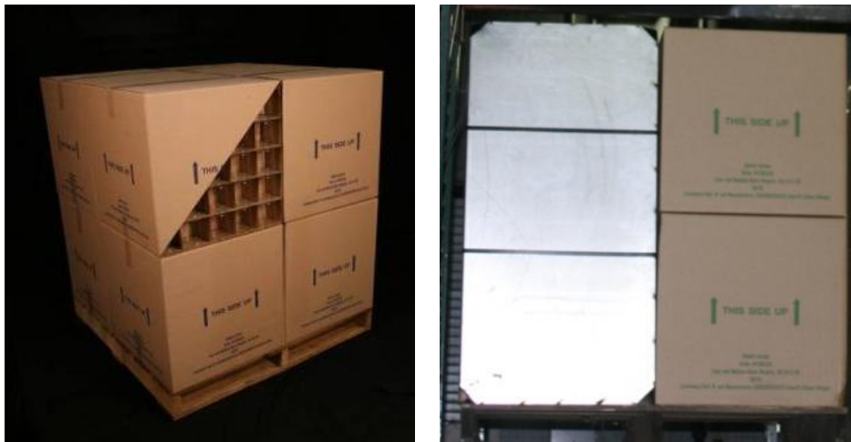
Figure 4-3: FM Global standard CUP commodity (left) and modified pallet design for reduced-commodity tests (right)
