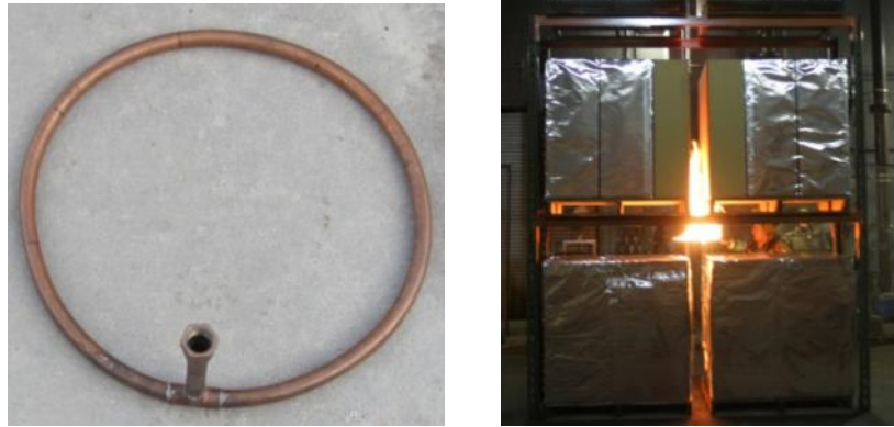
Figure 4-16: Propane ring burner (left) within the rack and fire size within rack (right)
