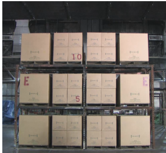
Figure 5-3: Rack storage array of cartoned unexpanded plastic commodity
