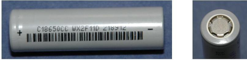
Figure 4-4: Li-ion cylindrical cell; external case side (left) and end view (right).
