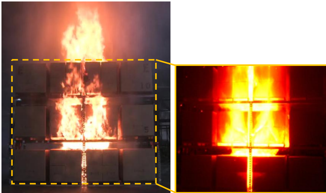
Figure 5-14: Image from HD camera (left) and IR camera (right) at first sprinkler operation [1 min 38 s] for Test 15
